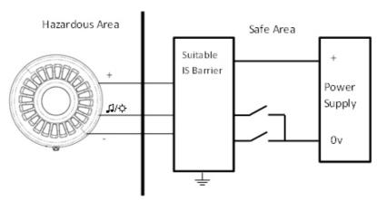
Switching between return paths will enable either Sounder or Beacon, alternately, both the paths could be activated to power both sections toaether.
